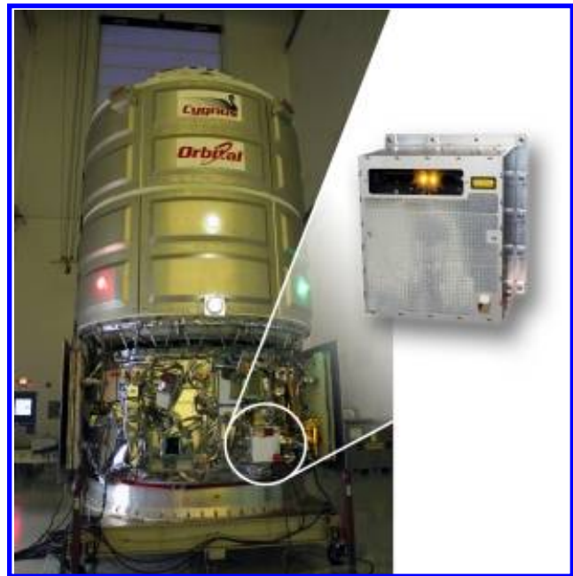
Figure 1. TriDAR installed on Orbital Sciences Cygnus spacecraft. Courtesy of Neptec Design Group Ltd.
